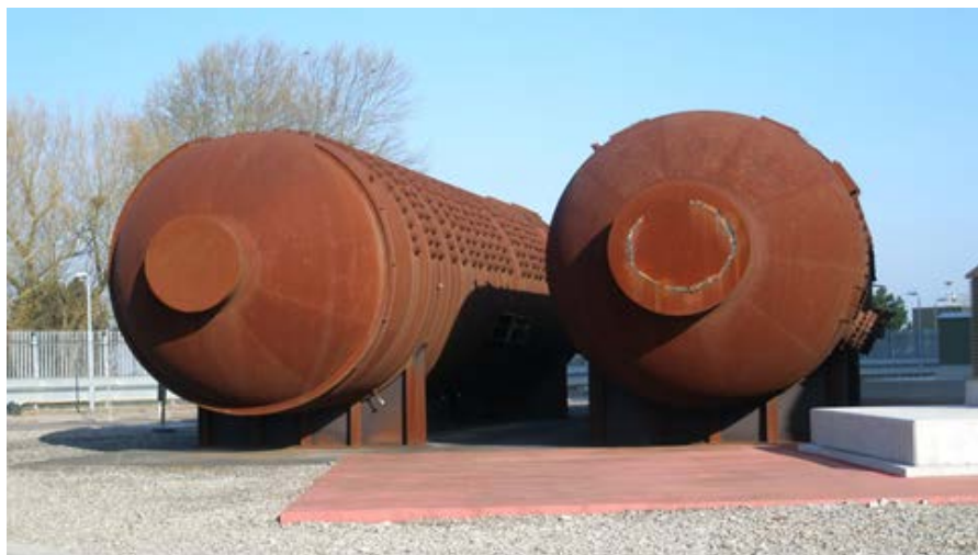
Fig. 3. Magnox Boilers (310 t each) for treatment.
